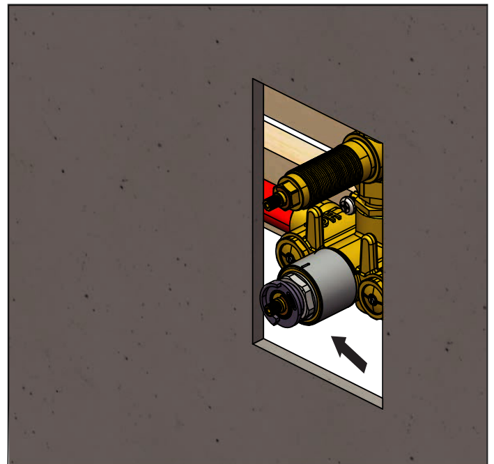
The 42mm ring must be flush. Otherwise the handle will not fit properly
